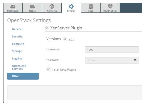
7. If the XenServer host already has compatible Nova plugins installed, untick the checkbox to install the supplemental packs. In normal cases, the XenServer host will not have compatible Nova plugins installed, so leave the checkbox enabled
