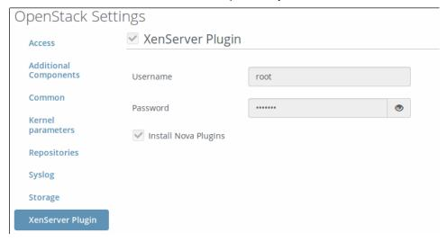
7. If the XenServer host already has compatible Nova plugins installed, untick the checkbox to install the supplemental packs. In normal cases, the XenServer host will not have compatible Nova plugins installed, so leave the checkbox enabled
